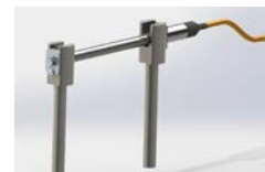
Extensometer (insensitive to temperature)
