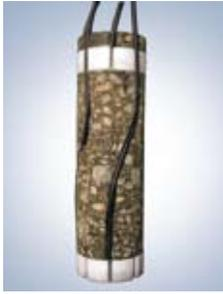
Composed of many different layers, each made with various materials, road structure is far from being a homogeneous platform. Each layer has its own role in the pavement structure and reacts differently under moving loads. To get the picture at different depth, Opsens has developed a multi-level fiber optic monitoring system to evaluate road behavior.
