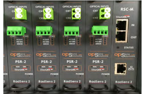
Two channels per module and two analog outputs
