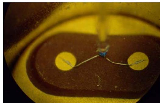
**Figure 5: Contact with bridge-wire**
