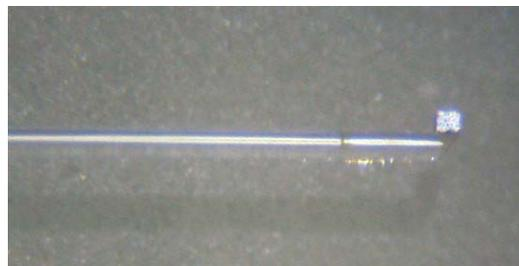
**Figure 8b: crystal mounted on the side of the optical fiber**
