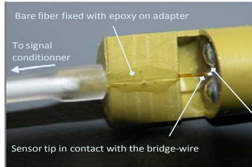
**Figure 6: Special adaptor designed to hold the sensor to the EED**
