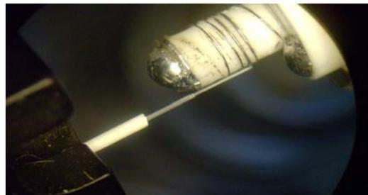
**Figure 8a: coiled bridge-wire**
