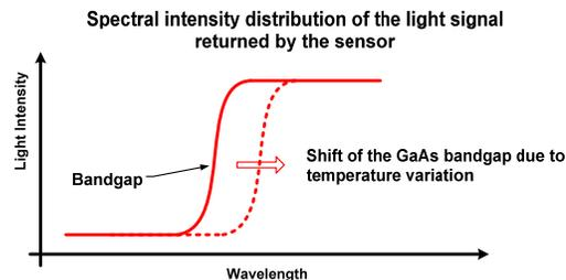
Figure 1: Schematic of the SCBG technology
